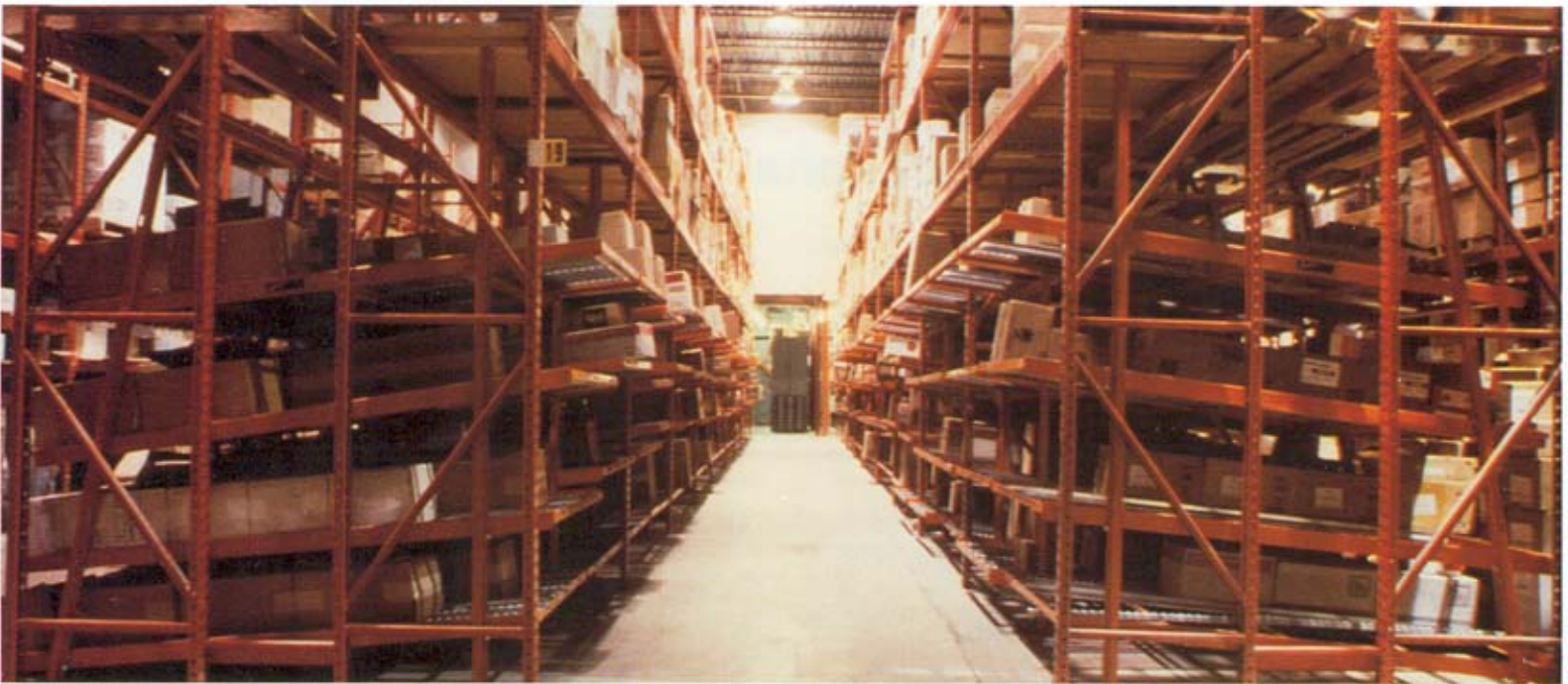
Lower levels of pallet racks house Keneco gravity flow systems, with replenishment in center aisle, order picking in outer aisles.
