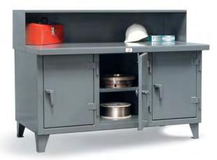
This workbench has three individual compartments and a riser shelf. The riser shelf is 12" high and 10" deep. Each individual compartment has an adjustable shelf and a three-point locking devise in each door.
