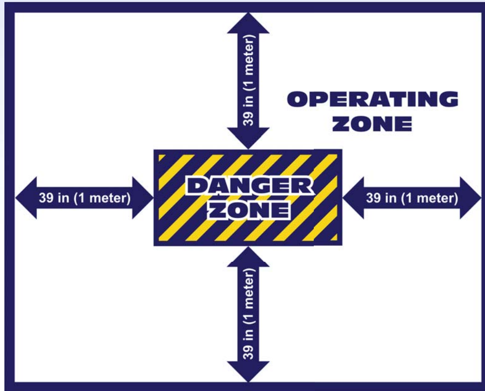
Figure 4 Recommended Floor Area
