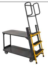
Ballymore introduces the heavy duty merchandise ladder cart with a capacity of 1,000 lbs. The cart has two large shelves for transporting a variety of merchandise. Ladder portion has a spring loaded device which secures the ladder to the floor when climbing and retracts for easy maneuvering. Cart is equipped with 4 casters- 2 swivels and 2 rigid for effortless turning and moving. Durable powder coated gray with yellow steps.
