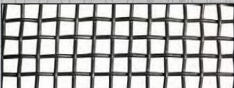
1/2" CENTER-TO-CENTER SQUARE 12 GAUGE WOVEN (3/8" SQUARE OPENING)
