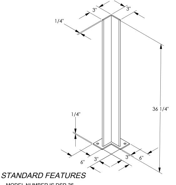
MODEL NUMBER IS DSP-36 OVERALL WIDTH IS 6" OVERALL LENGTH IS 6" OVERALL HEIGHT IS 36 1/4" BASE PLATE: 1/4" X 6" X 6" MOUNTING HOLES: (3) - Ø9/16" GUARD ANGLE: 1/4" X 3" X 3" Hot Rolled Steel
