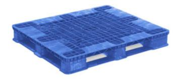
It is manufactured of high-density polyethylene and will edge-rack up to 750 pounds. The smooth, non-porous construction protects product (no nails, rust or splinters) and does not absorb moisture or odor. Its all-plastic construction ensures dimensional consistency and repeatable performance during its entire service life. The open, flow-through design creates a hygienic solution for food/agricultural applications. Available in blue. NOTE: Pictured with optional stringer.
