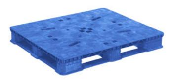
It is manufactured of high-density polyethylene and will edge-rack up to 2100 pounds. The smooth, non-porous construction protects product (no nails, rust or splinters) and does not absorb moisture or odor. Its all-plastic construction ensures dimensional consistency and repeatable performance during its entire service life. The solid deck creates an alternative hygenic solution for customers who do not have pallet washers. Available in blue.
