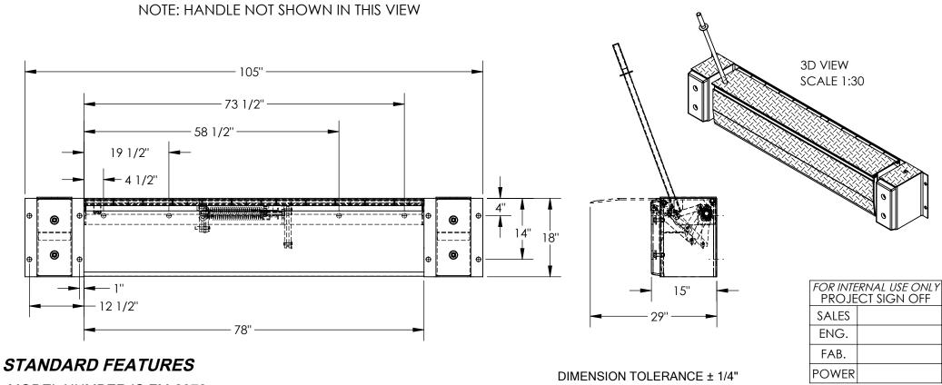
**MODEL NUMBER IS FM-2078 DECK WIDTH IS 78" OVERALL WIDTH IS 105"** MAX CAPACITY IS 20.000 LBS. STANDARD TOE GUARDS **GREASE ZERK FITTINGS** 18" HIGH BUMPERS (TO SERVE LOW TRUCKS) ADJUSTABLE TORSION SPRING COUNTERBALANCE MECHANISM SERCIVE RANGE OF 5" ABOVE AND BELOW DOCK UNIT COMES WITH HANDLE AND BUMPERS TREADPLATE RAMP & DECK CONSTRUCTION DURABLE LIQUID PAINT BROWN FINISH
