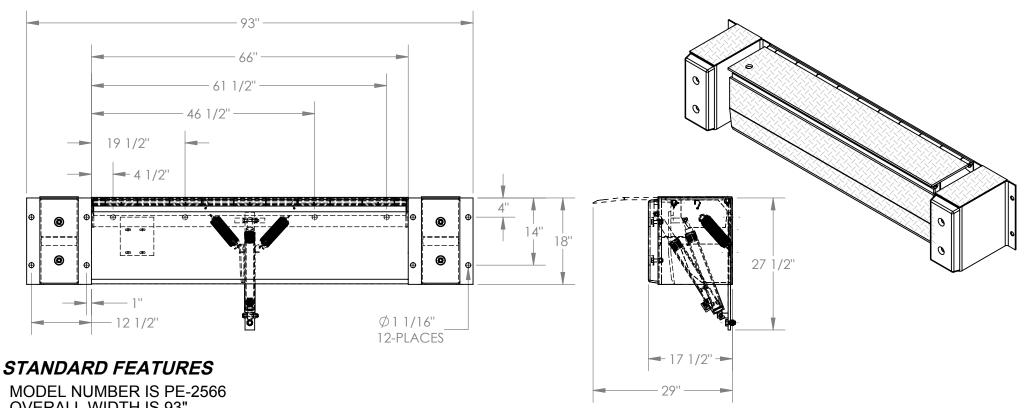
**OVERALL WIDTH IS 93" DECK WIDTH IS 66" OVERALL DEPTH WITH RAMP OUT IS 29" BUMPER PROJECTION IS 17 1/2"** UNIFORM CAPACITY IS 25,000 lbs. 5" ABOVE / 5" BELOW SERVICE RANGE RECOMMENDED FOR DOCKS AT LEAST 48" HIGH. UNIT COMES WITH MOTOR, PUMP, CONTROL BOX, CYLINDER. HYDRAULIC LINES AND OIL. TREADPLATE RAMP & DECK CONSTRUCTION
