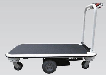
The Moto-Cart Electric Platform Truck (MC) is a DC-powered self-propelled cart with a two-wheel drive and four casters. This flexible vehicle can travel over carpeting, tile, hard surfaces, and in and out of elevators. The MC is available in various capacities and platform sizes and has an internal trans-axle drive system that allows the cart to rotate.
