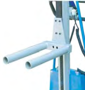
Attachment A-3 is a dual ram arrangement. The ram length is 17.75" long and 2" in diameter. The distance between the rams is 6". It can be used to cradle rolls or can handle two small rolls at one time through the core.
