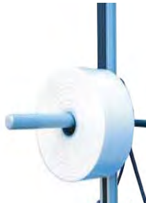
Attachment A-2 is a single ram suited for lifting coils or rolls through the core. The ram length is 24" long and 2" in diameter.
