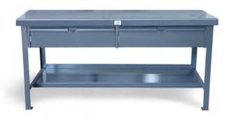
These shop tables are ideal for assembly, packing, shipping, maintenance or wherever a large working area is required. The legs are  $2'' \times 2'' \times 1/4''$  angle and the top is 7-gauge steel with a  $1\,3/4''$  maple block attached. Both drawers are 6'' high, 20'' in depth, have a hasp for a padlock, and can hold up to 400 pounds. Construction is all-welded to give superior rigidity and stability. Additional table top options on page 111.
