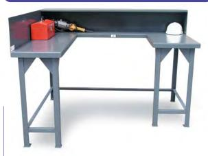
This custom shop table has an overall width of 72", varying depths of 9", 36", and 56", with a height of 38" and an overall height of 50". There is no bottom shelf, instead heavy duty angle is used for strength and rigidity. Unit also features a 7-gauge top, riser shelf and side guard.
