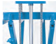
Twin heavy duty lifting chains provide a 2:1 lifting ratio for shorter lift stroke and reduced cylinder wear.
