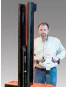
Narrow mast and offset design provide workers a clear view with no blind spots.
