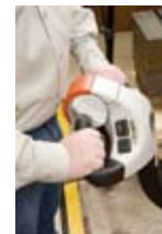
Auto-reversing "belly bump" switch protects against operator accidents while working in tight quarters.
